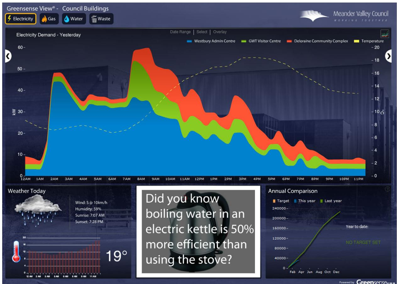
Figure 1: The screenshot above reveals the electricity usage for the 3 buildings, over a 24 hour period; the weather; a tip for saving money; and a comparison of the current years energy use to the previous year.
