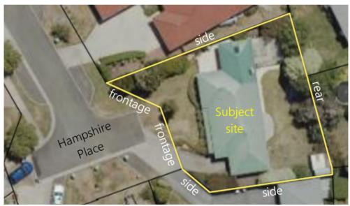
Figure 2: Aerial image showing allocation of boundaries (source: Spectrum Spatial).
