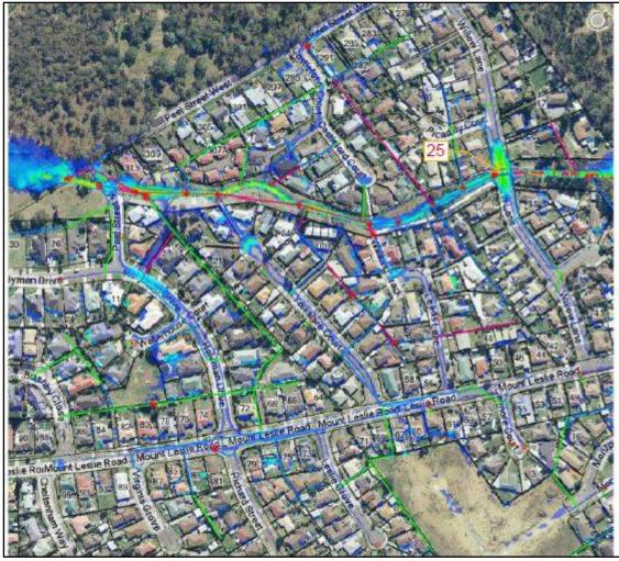
Figure 10. North Prospect Vale – Willow Lane Stormwater System 1% AEP.
