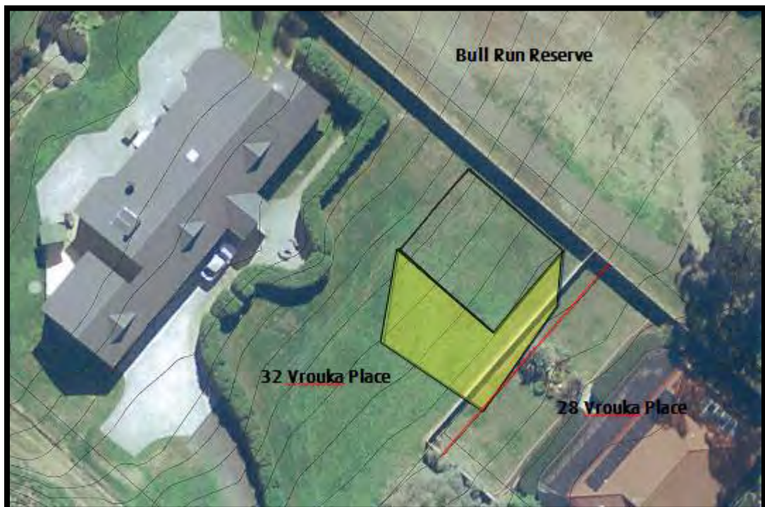
Photo 3: Showing approximately the 12 noon shadow (yellow area) from proposed outbuilding The red line shows the potential shadow from a 2.1 m high fence Contour lines are 0.5m intervals
