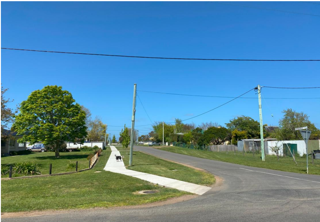
Figure 5: Ashburner Street, typical example of the narrow carriageway, grassed swales and European/exotic street tree (Source: David Cundall)
