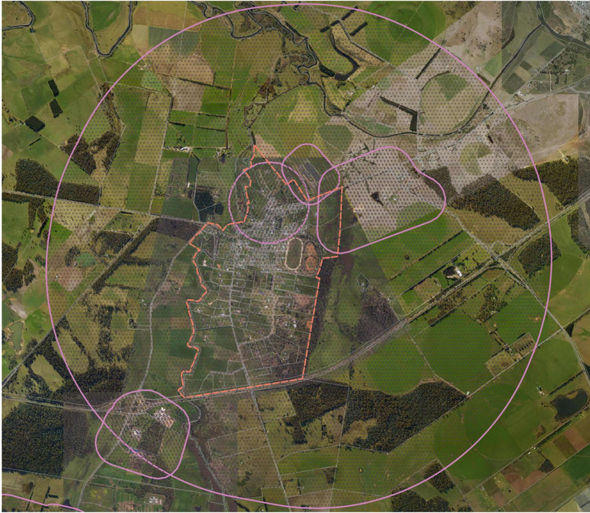
Figure 13: Attenuation Buffers of known attenuating activities within the investigation area source: adapted from the LIST)
