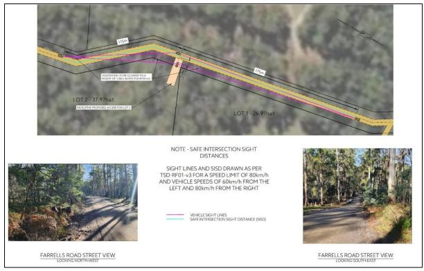
Figure 3 - Excerpt of the TIS showing the location of the proposed new vehicle crossing and location of vegetation required to be cleared within the road reserve.
