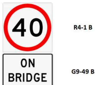
Figure 23 – Suggested Wadleys Road Bridge speed limit.
